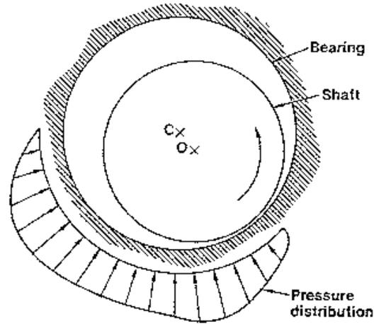
**Fig. 2: Hydrodynamic Pressure Generation**
