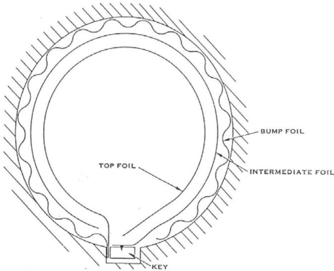
**Fig. 4: Reversed Multilayer Foil Journal Bearing Schematic**
