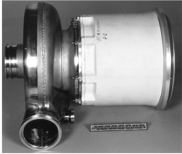
**Fig. 24: B-2 Foil Bearing Air Cycle Machine**
