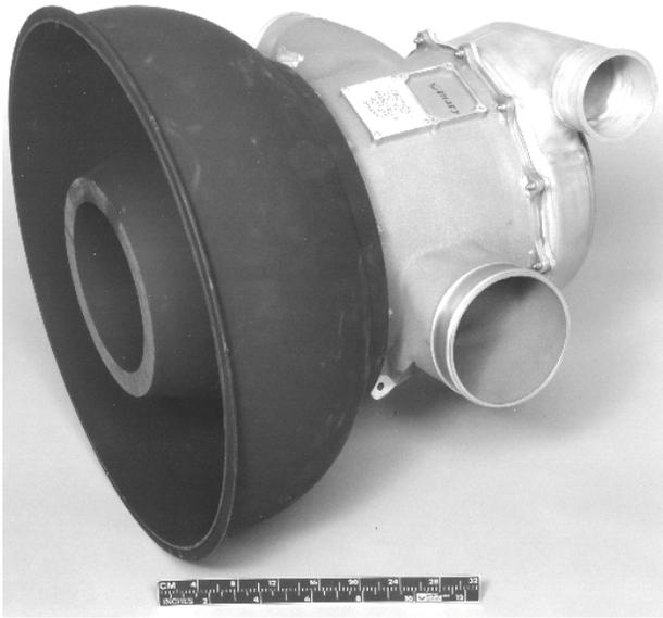
**Fig. 22: 747 Foil Bearing Air Cycle Machine**
