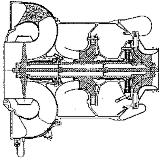
**Fig. 20: L-1011 Foil Bearing Air Cycle Machine**
