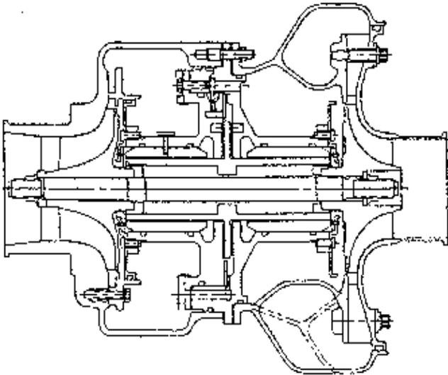
**Fig. 23: B-1B Foil Bearing Air Cycle Machine**
