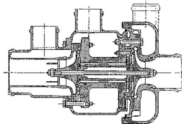
**Fig. 15: Cessna-550 Foil Bearing Air Cycle Machine**
