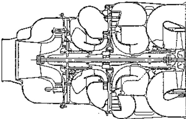
**Fig. 27: 777 Foil Bearing Air Cycle Machine**
