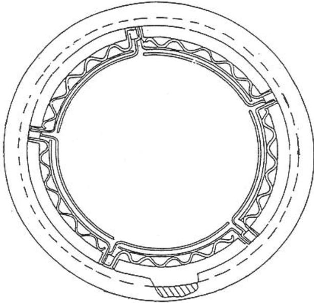
**Fig. 7: Reversed Multipad Foil Journal Bearing Schematic**
