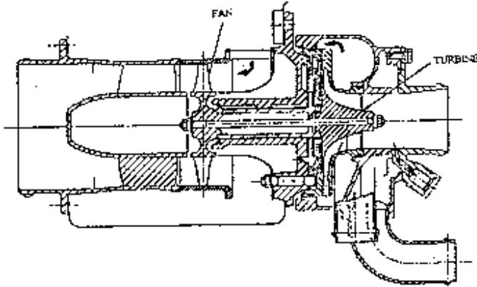
**Fig. 19: M1A1 Tank Foil Bearing Air Cycle Machine**
