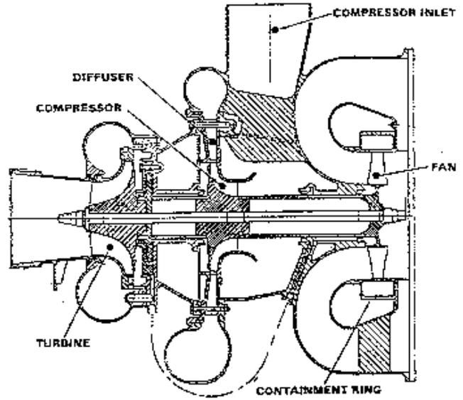
**Fig. 17: 767/757 Foil Bearing Air Cycle Machine**
