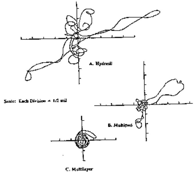
**Fig. 6: Orbits of Various Foil Journal Bearings under 27 lbs. of Shock Load**
