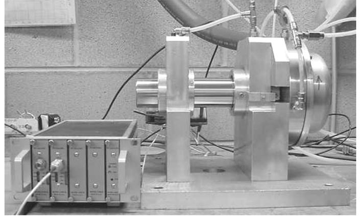
**Fig. 10: Journal Bearing Test Rig**
