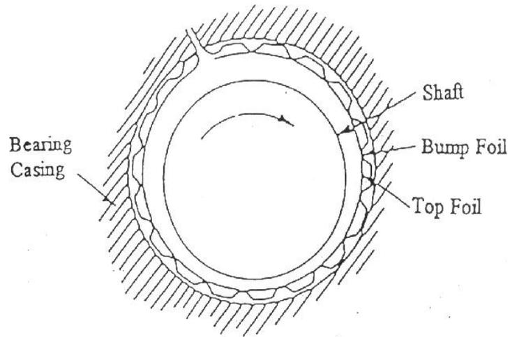
**Fig. 5: Hydresil Foil Journal Bearing Schematic**
