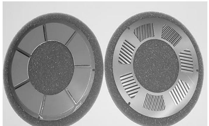
**Fig. 9: Dual Spring Foil Thrust Bearing**
