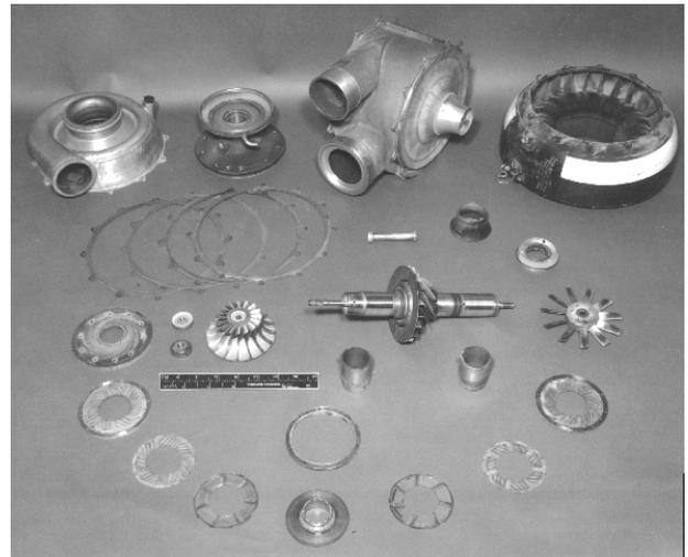
**Fig. 21: L-1011 Foil Bearing Air Cycle Machine**
